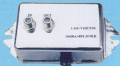
PT-201 BANDWIDTH:45-750MHZ MAX GAIN:10DB OUTPT:1WAY 75Ω
