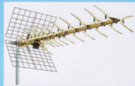
FREQUENCY RANGE: 470-862MHZ RECEIVING RANGE: UHF GAIN: 14DB OUT IMPEDANCE: 75Ω STANDING WAVE RATIO: \leq 1.5 DB
