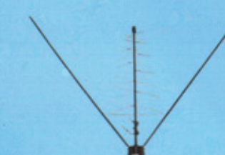
H3311 FREQUENCY RANGE:47-862MHZ VHF/UHF GAIN: 9DB CHANNEL 1-5 (VHF I 47-108MHZ): 0 DB CHANNEL 6-12 (VHF II 174-230MHZ): 1 DB CHANNEL 21-60 (UHF 470-862MHZ): 9 DB OUT IMPEDANCE: 75Ω STANDING WAVE RATIO(SWR): ≤1.6DB WEIGHT: 1.7 KG
