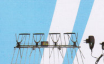
SYN-005/0DX FREQUENCY RANGE: 470-862MHZ UHF CHANNEL: 21-60 GAIN: 15-25DB OUT IMPEDANCE: 75Ω STANDING WAVE RATIO(SWR): ≤1.6DB POWER SUPPLY: 12V/100MA ASSEMBLED WITH AMPLIFIER SWA SERIES WEIGHT: 1.3 KG
