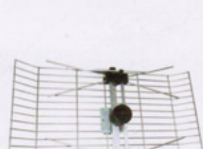
SYN-006/1DX FREQUENCY RANGE: 470-862MHZ UHF CHANNEL: 21-60 GAIN: 10-12 DB OUT IMPEDANCE: 75Ω STANDING WAVE RATIO(SWR): ≤1.5DB WEIGHT: 0.95 KG
