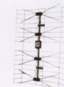
A1001/0DX FREQUENCY RANGE: 470-862MHZ CHANNEL: 21-60 GAIN: 12-15DB OUT IMPEDANCE: 75Ω STANDING WAVE RATIO(SWR): ≤1.5DB POWER SUPPLY: 12V/100MA ASSEMBLED WITH AMPLIFIER SWA SERIES WEIGHT: 1.5 KG
