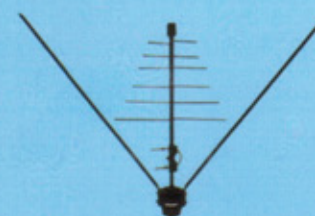
H321 FREQUENCY RANGE:47-862MHZ VHF/UHF GAIN: 10 DB CHANNEL 1-5 (VHF I 47-108MHZ): -0.5 DB CHANNEL 6-12 (VHF II 174-230MHZ): 0.6 DB CHANNEL 21-60 (UHF 470-862MHZ): 10 DB OUT IMPEDANCE: 75Ω STANDING WAVE RATIO(SWR): ≤1.5DB WEIGHT: 1.1 KG
