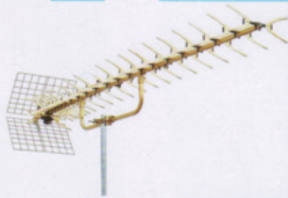
U-24X FREQUENCY RANGE: 470-862MHZ RECEIVING RANGE: UHF GAIN: 18DB OUT IMPEDANCE: 75Ω STANDING WAVE RATIO(SWR): \leq 1.5 DB
